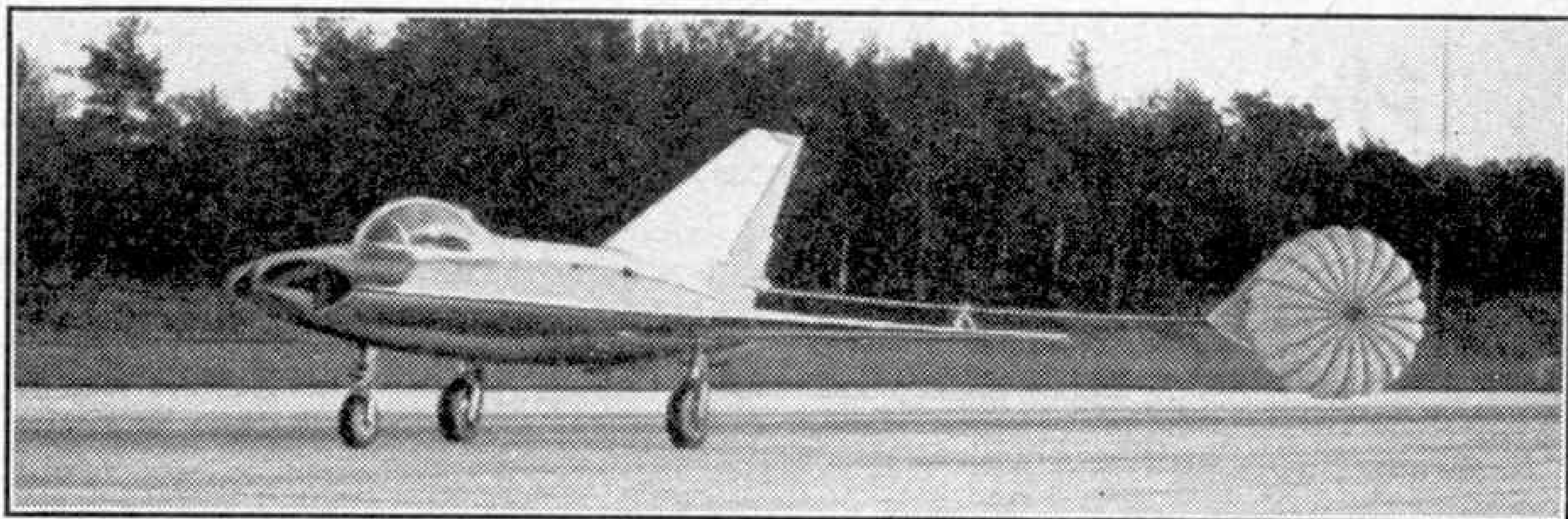
Saab 210 Draken, the first Swedish delta-wing jet aircraft. Note the special drag parachute to reduce the landing run. Photograph by courtesy of Svenska Aeroplan A.B., Sweden.
