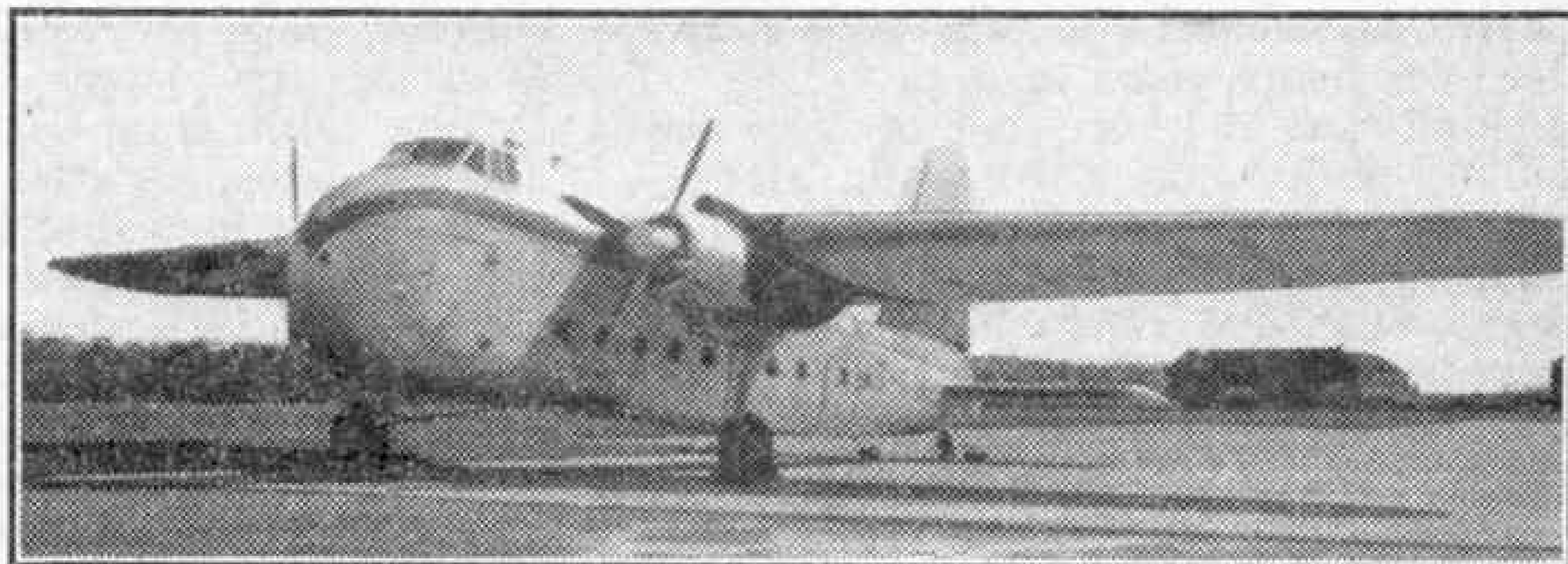
This view of the aircraft with its nose-doors closed gives a good idea of the great width and depth of the cargo-hold. Photograph by R. Knight, Winchester.
