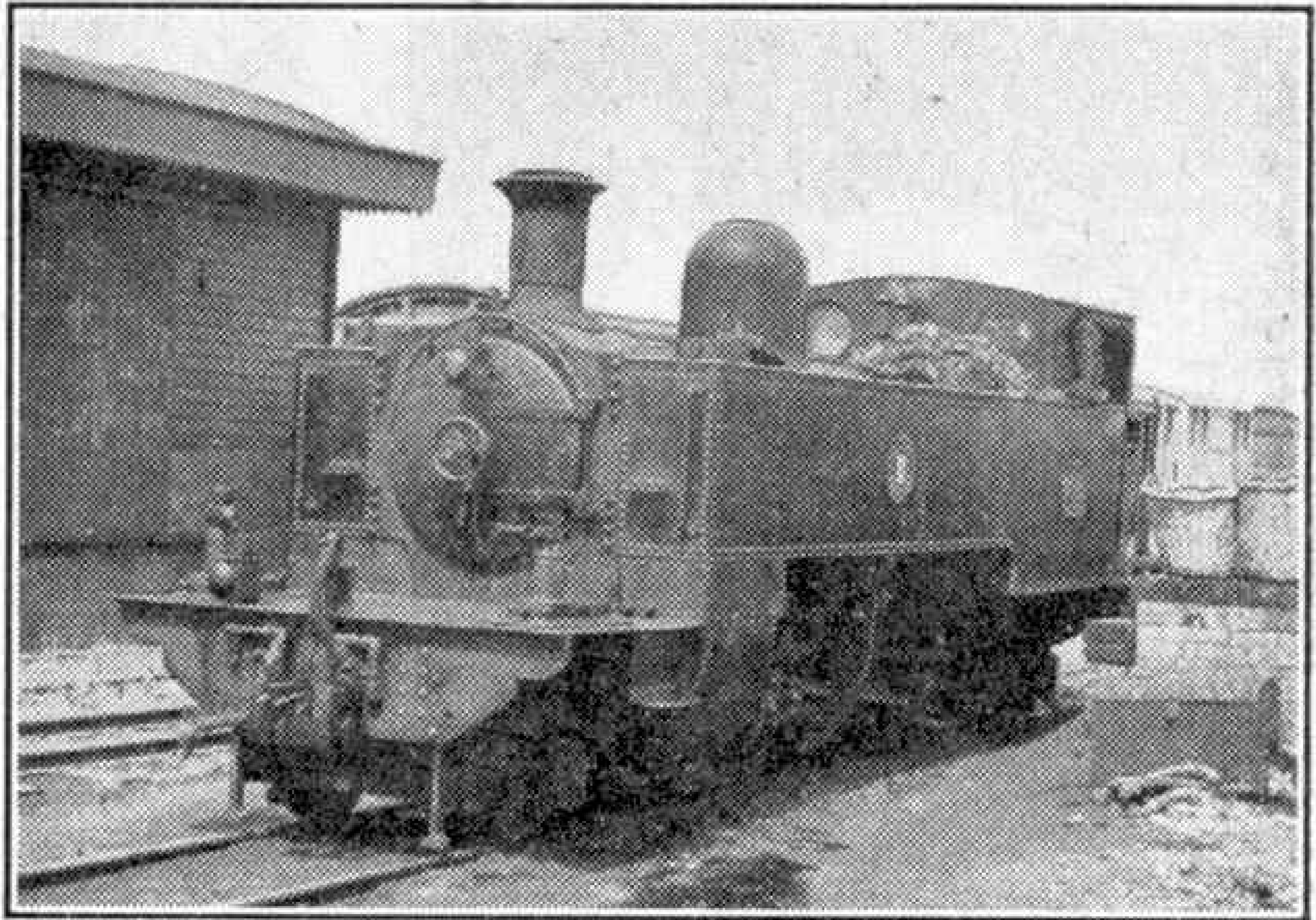
Engine No. 44 of Class "S" at the coaling stage at Ballymoney. Note the coal baskets on the raised platform.
