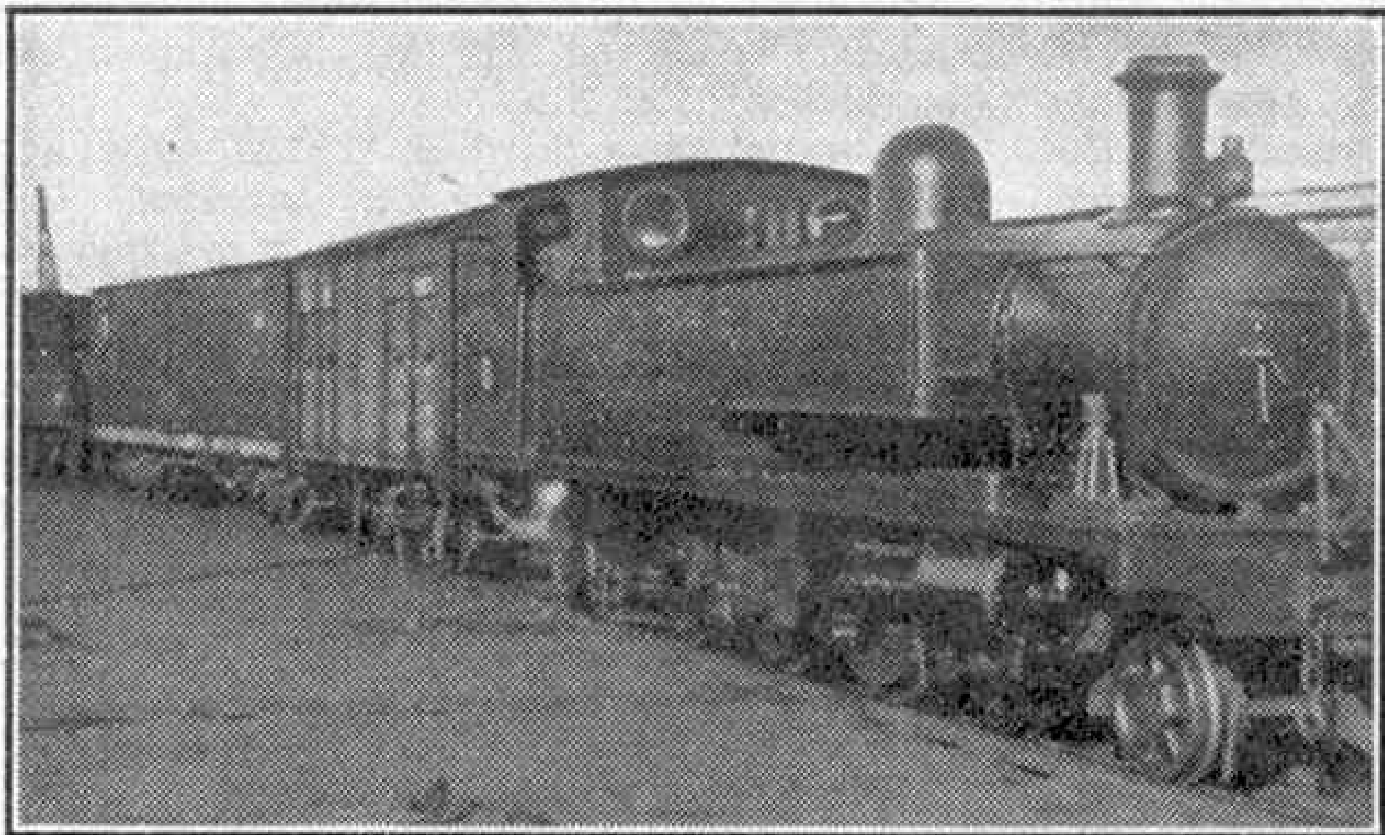
County Donegal steam power is represented by this picture of one of the 4-6-4 tanks. Photograph by courtesy of County Donegal Railways.
