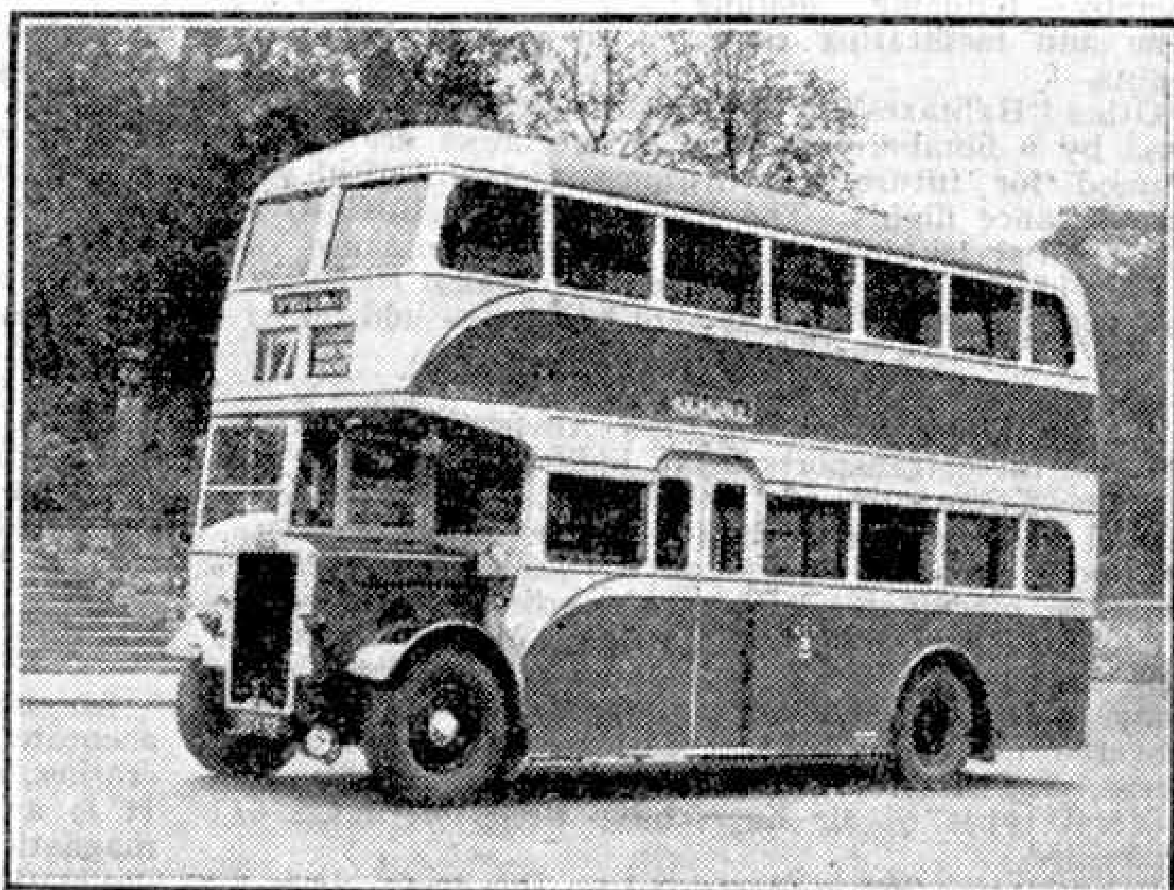
A new Leyland bus of the Rochdale Corporation that has been fitted with sliding doors.
