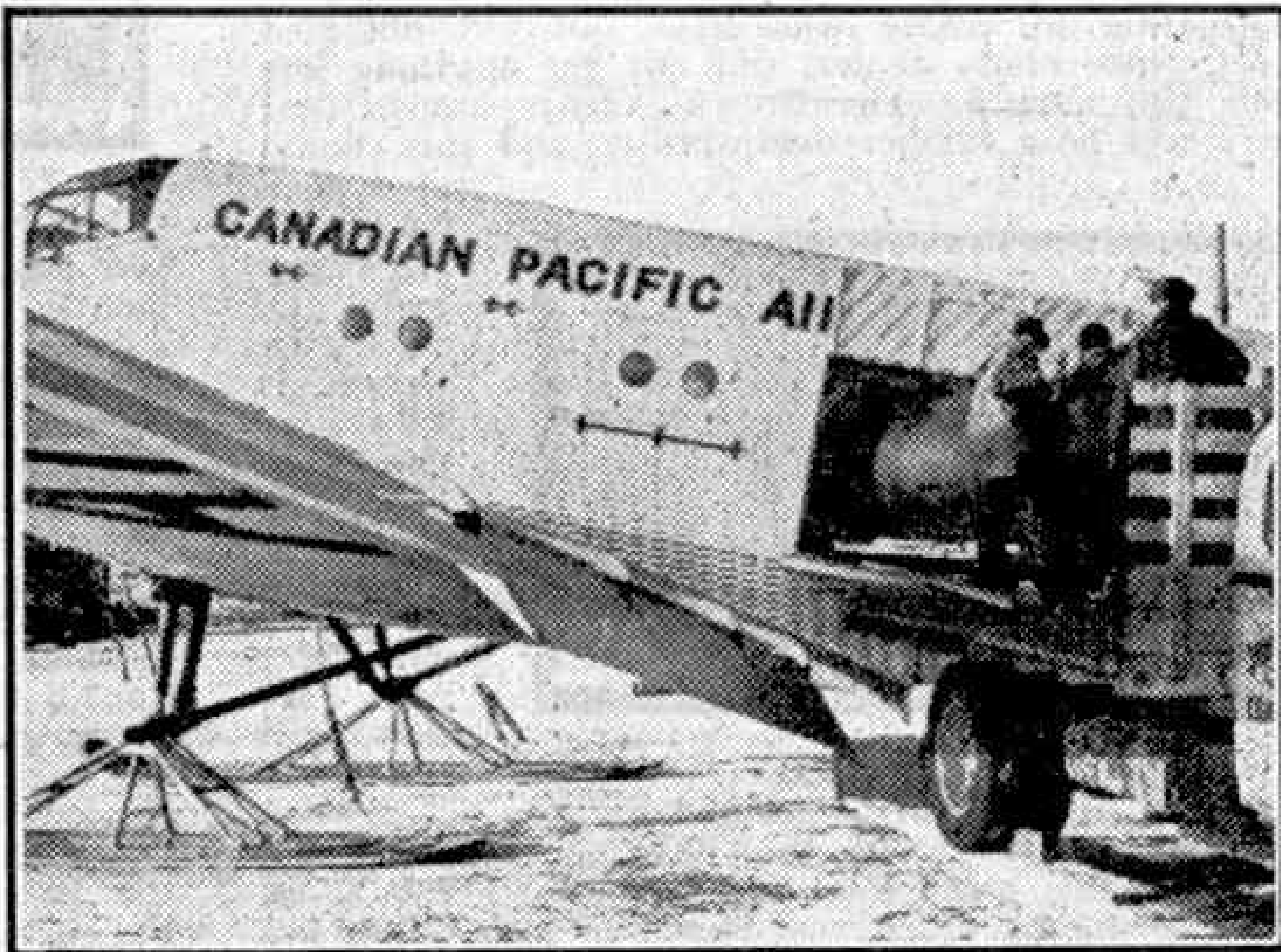
Loading a 2,700 lb. boiler, destined for a cobalt mine in Ontario, into the fuselage of a Canadian Pacific Air Lines freight transport machine. Canadian Pacific photograph.
