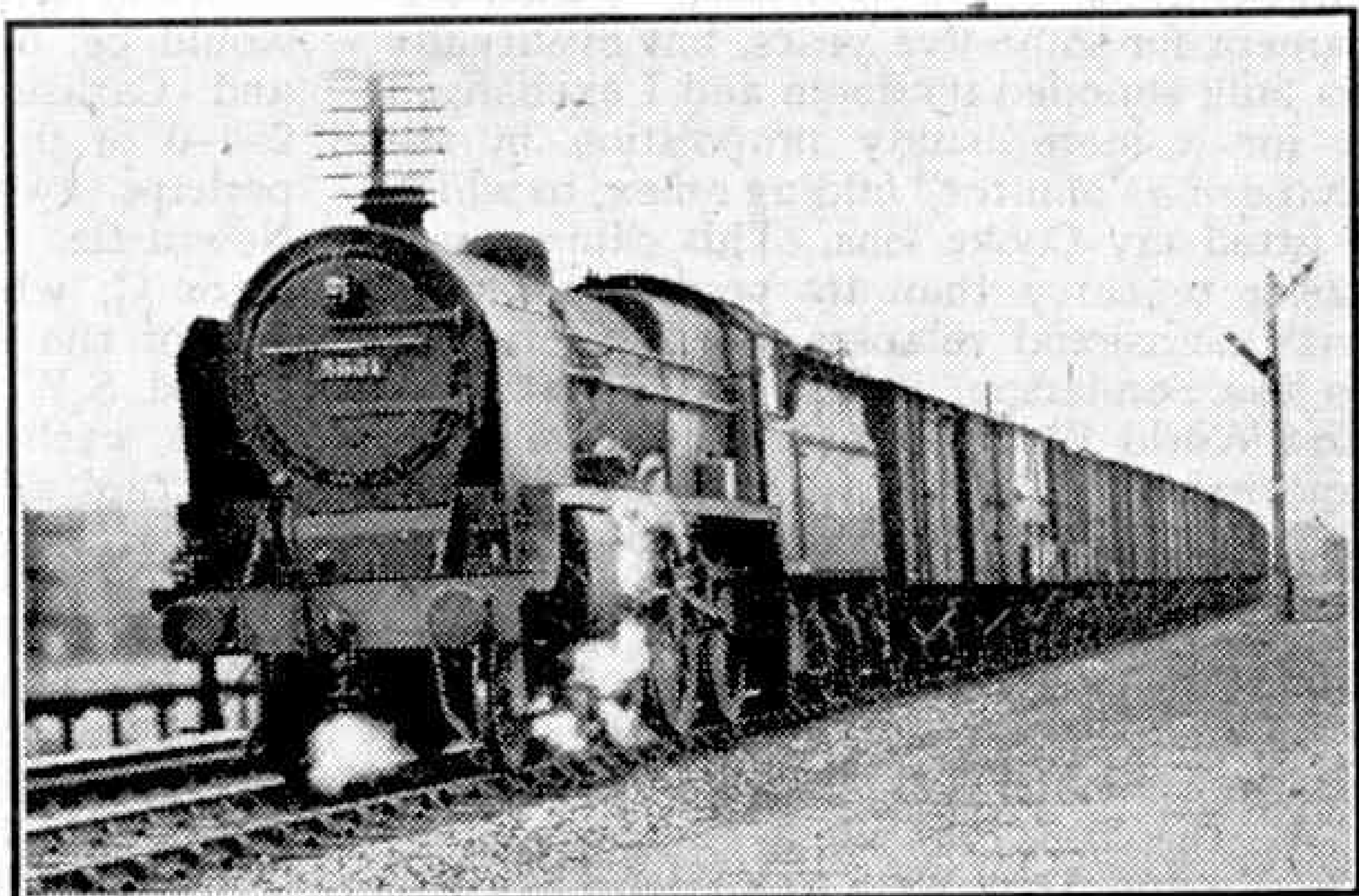
An express passenger engine in fast goods service. An L.M.S. "Patriot" class 4-6-0 No. 5531 on the pre-war 11.25 a.m. express goods from Camden. Photograph by courtesy of the L.M.S.R.
